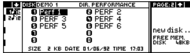
Directory of the Performances contained in a Bank/Song. You can return to the Bank/Song directory with the left multifunction button.
