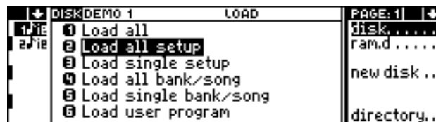
“Load all Setup” is shown selected. A Bank/Song Group number is not shown because the disk (and memory) can contain only one Setup of each type.
